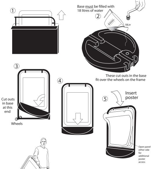
Once assembled, the whole sign can be easily moved without the need to remove the base.
